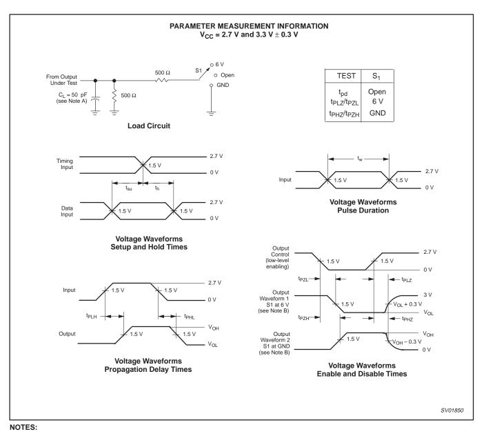
A. CL includes probe and jig capacitance.
