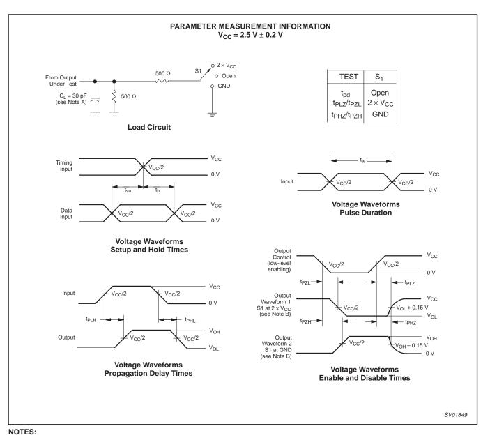
A. CL includes probe and jig capacitance.
